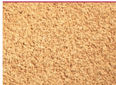
Alm. Borebille - boremel. (Foto: Protox)
