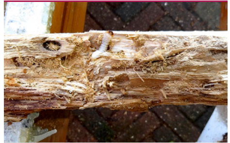
in 15 Red-brown Longhorn Beetle - larva, frass and decomposed wood. (Photo: Protox/customer photo)
