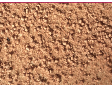
i 3 House longhorn beetle – frass with characteristic wine cork-shaped excrement. (Photo: Protox/Goritas)
