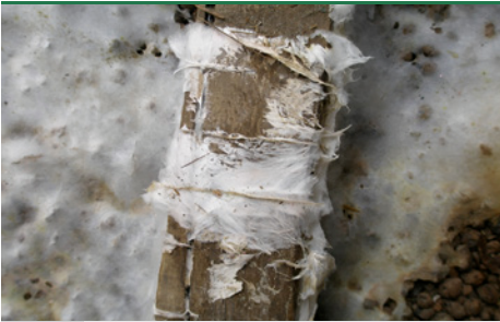
svn 27 Dry rot fungus - young mycelium with string formations, slatted in conservatory. (Photo: Protox)
