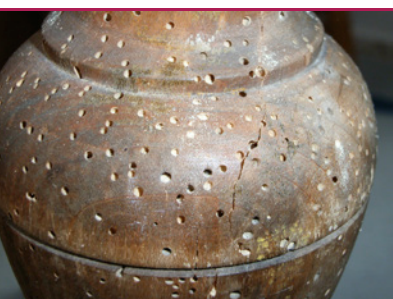
i 10 Common furniture beetles - exit holes in table legs. (Photo: Prottox)
