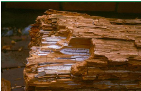
Mine fungus - decomposition and white surface mycelium on fracture surfaces. (Photo: Goritas)
