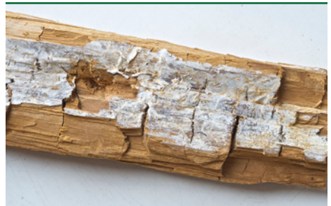
Mine fungus - white surface mycelium on decomposed wood with fissure blocks. (Photo: Protox/Goritas)
