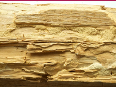
i 2 House longhorn beetle – exposed larval passages with frass. (Photo: Protox/Gorita's archive)
