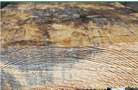
Blue stain fungus - attacked softwood in pith rays from the surface to the core of the tree. (Photo: Prottox)
