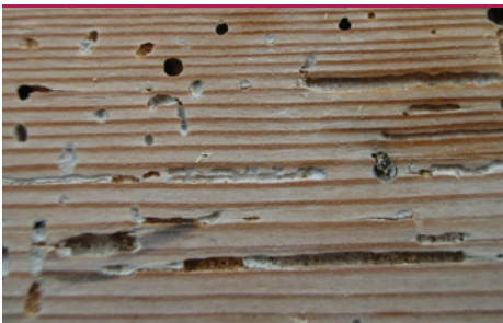
in 16 Common furniture beetles in floorboard - exit holes and larva passages exposed due to planing. (Photo: Protox)
