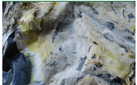
svn 30 Dry rot fungus - surface mycelium with characteristic yellow spots. (Photo - Protox)
