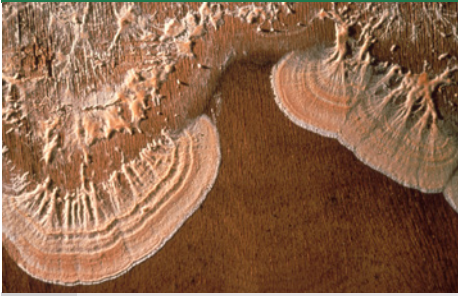
svn 37 Gilled polypore – surface mycelium in a flat roof made of plywood. (Photo: Protox/Gori)
