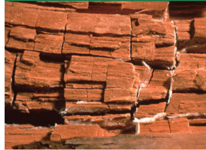
Brown rot - the fungus breaks down the cellulose fibres, leaving the lignin.
