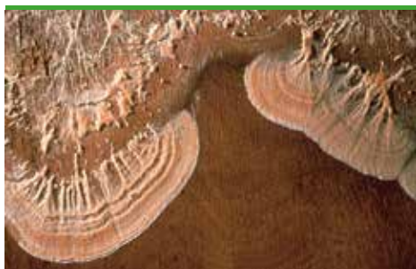
svn 37 Korkmussling - ytmycel i platt plywoodtak (foto - Protox/Gori A/S)
